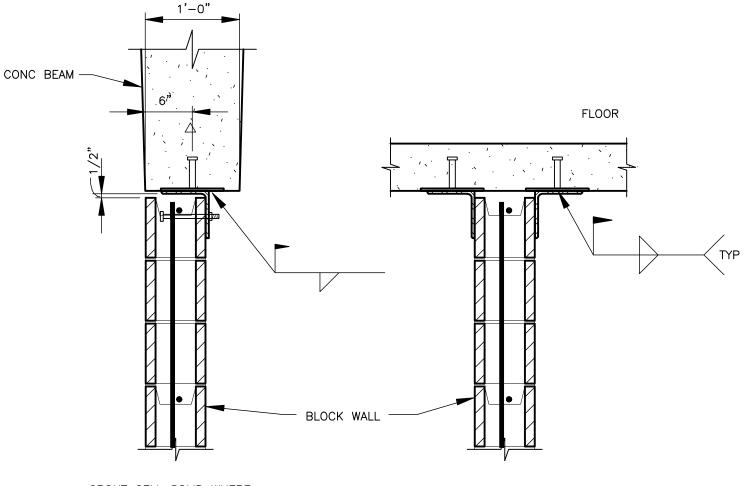
GROUT CELL SOLID WHERE ANCHOR BOLT OCCURS
