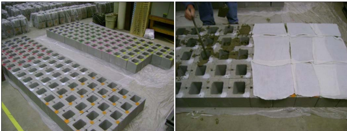
Figure 2: CMUs Prior to Casting Grout Samples and Grout Samples During Casting
