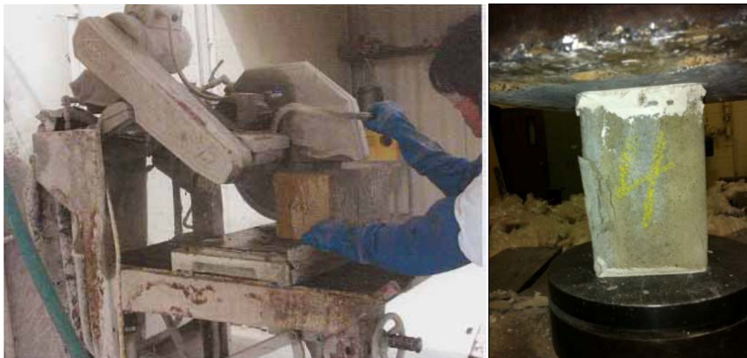
Figure 3: Saw-Cutting of a Grout Specimen and Grout Sample During Testing
