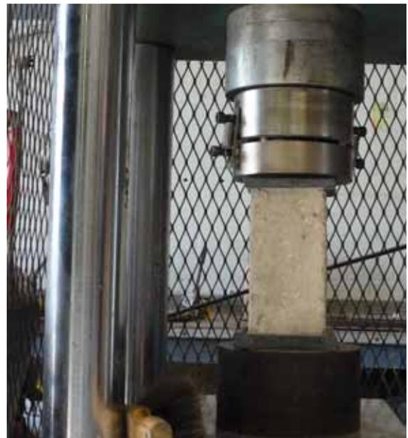
**Figure 3: Compression Testing of Grout Specimen**
