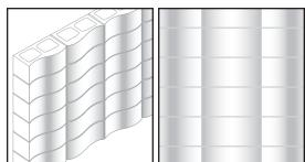
The Pixel Blocks are manufactured in Precision texture. Note: base dimensions and core alignments are intended for 8x8x16 design modules. Consult your Angelus representative for detailing.
